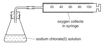
Sodium chlorate(I) is placed in the flask and  $0.2\,g$  of copper(II) oxide is added. This catalyses the decomposition of the sodium chlorate(I) and the volume of oxygen collected is measured every minute. The results are plotted to give a graph of the type shown below.
